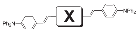
FIGURE 2. General OPV structure where X denotes the moiety in which systematic molecular changes were made.
